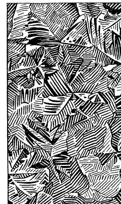
FIG. 2.—SPANGLES ON SURFACE OF GALVANIZED SHEET IRON
